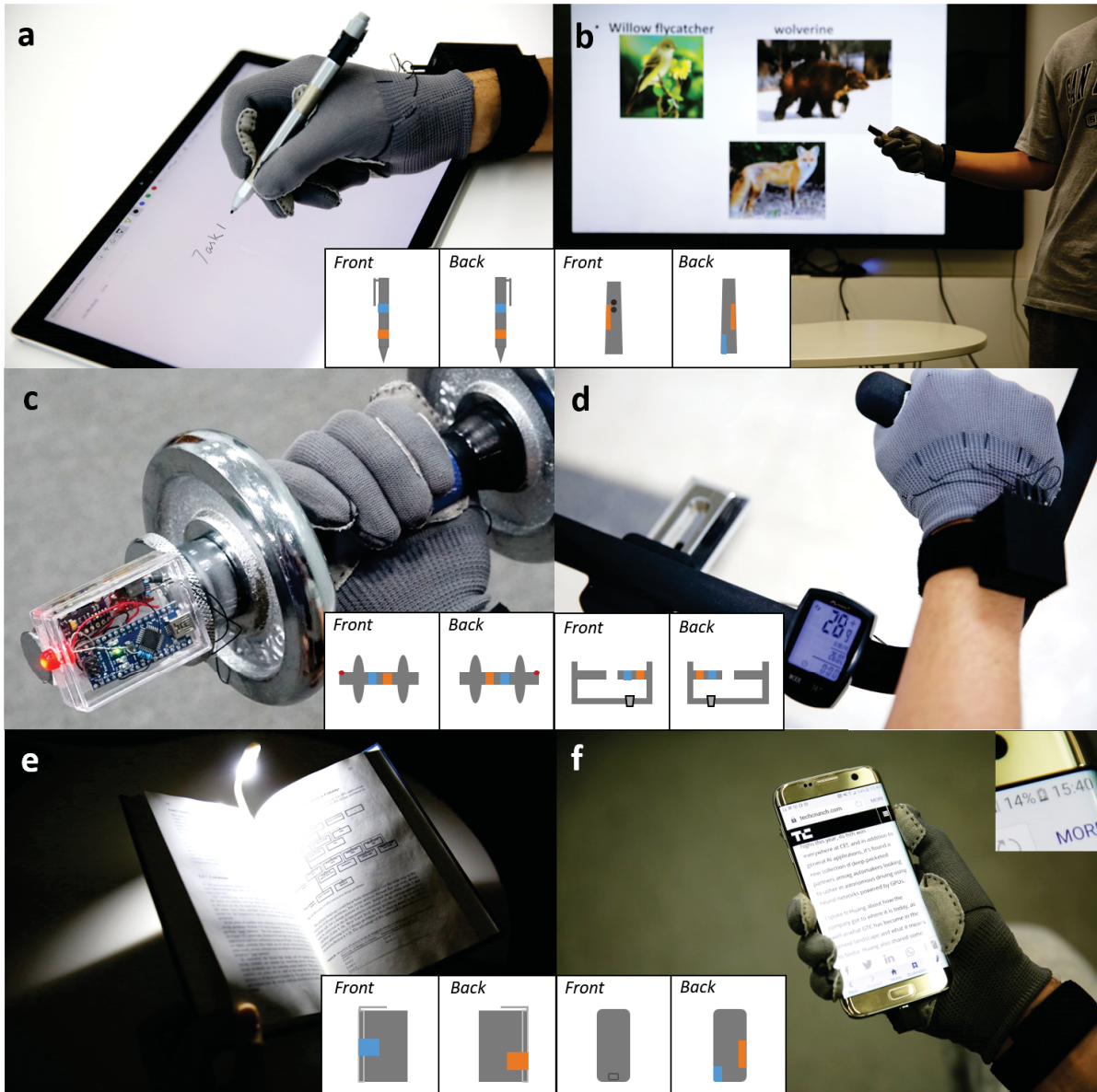
Fig. 7. Applications for TouchPower. Two electrodes (shown in blue and orange) are applied to each device. All electrodes are made from conductive tape. We show TouchPower used in an office setting with a stylus (a) and a presentation remote controller (b), as well as in a gym setting with a dumb-bell (c) and a gym bike (d). TouchPower can also light a book (e) and charge a cellphone (f). We zoom in to show the charging status on the top right corner of (f).
