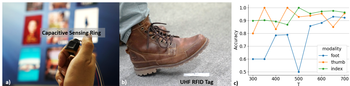
Fig. 11. The participant can tap the thumb on a ring (a) or tap a foot on a UHF RFID tag (b) to select on-screen objects. The selection accuracy for different modalities with respect to target pattern period using Correlation recognizer is also shown (c). We added the index data from Study 2 for comparison
