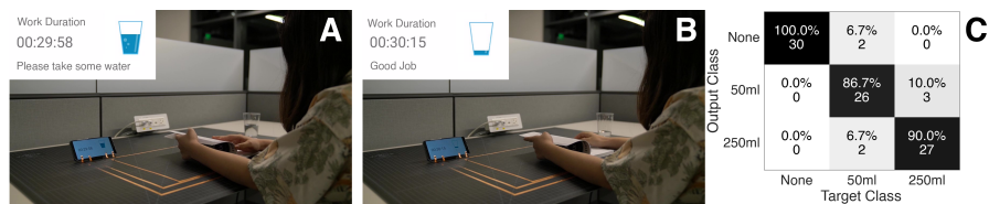
Fig. 12. Smart desk example detecting user and object’s presence and status
